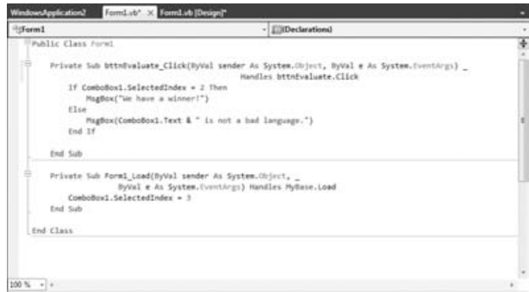
FIGURE 1.9 Outline of a subroutine that handles the Click event of a Button control
