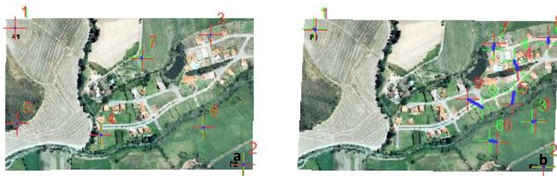
Figure 9. Distribution of control points: (a) homogeneous distribution, and (b) heterogeneous distribution
