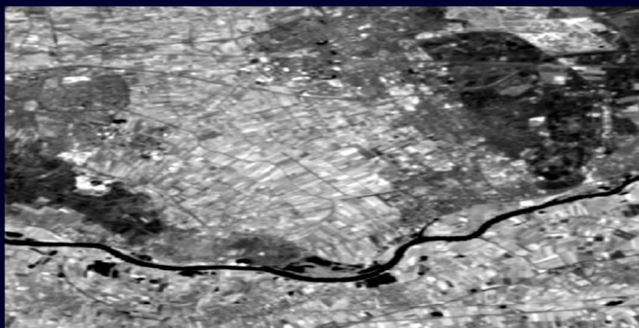
Result low pass filter, 3x3 window
