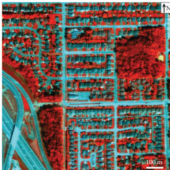
FIGURE 1.5 Color composite image created from CASI-1500 VNIR hyperspectral bands acquired in Surrey, BC, Canada, in May 2013. Band 70 (1.0273 \mu\text{m} ) is used as red, band 15 (0.5020 \mu\text{m} ) as green, and band 5 (0.4061 \mu\text{m} ) as blue.
