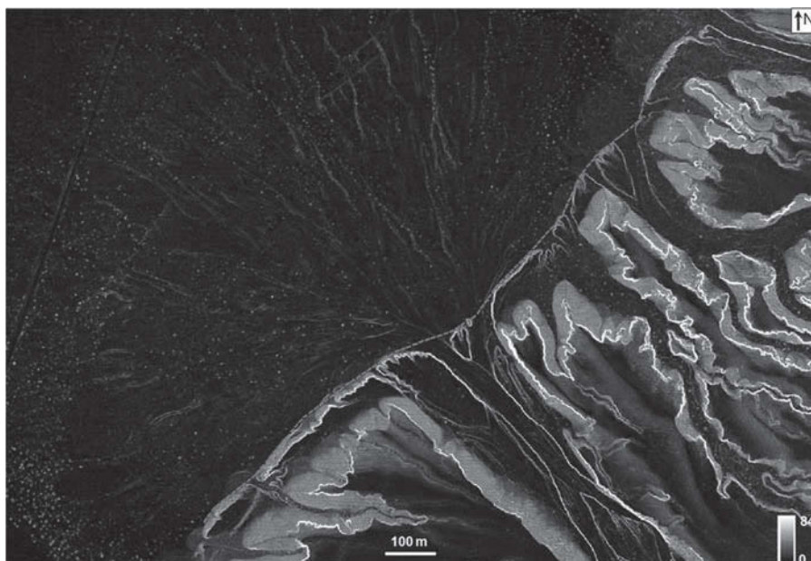
FIGURE 6.24 Slope raster created from 1-m resolution LiDAR-derived DEM of Willow Valley in Death Valley, CA (USA).
