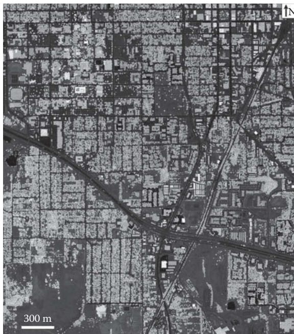
FIGURE 5.4 A merged image is created by adding LiDAR intensity image and non-ground DSM.
