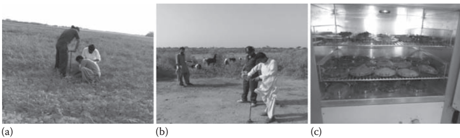
FIGURE 13.2 (a and b) Field sample collection using soil auger. (c) Samples in the laboratory oven.
