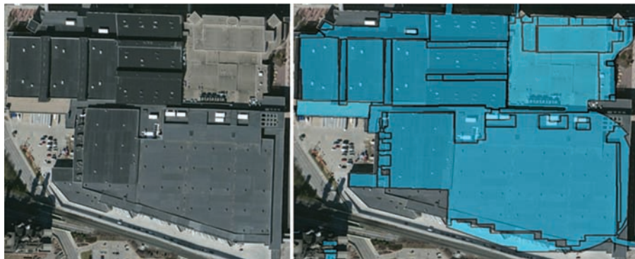
FIGURE 17.2 Step edge detection on a building roof.
