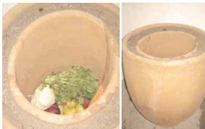
Figure 6: An evaporative cooler
