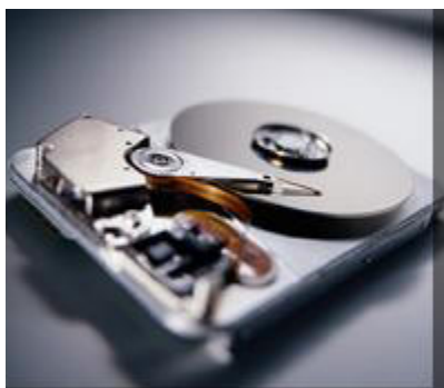
Read/Write Heads and Spindle Motor
