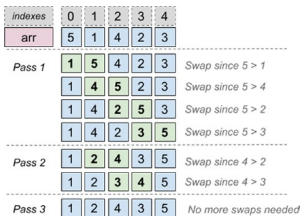
Figure 7-7. Bubble sort phases and effect
