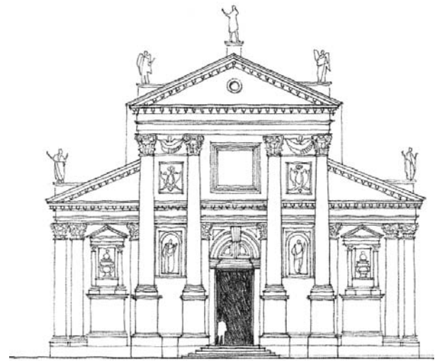
S. Giorgio Maggiore , Venice, 1566–1610, Andrea Palladio. Facade completed by Vincenzo Scamozzi. The entrance facade operates at two scales: that of the building as a whole facing a public space and another at the size of a person entering the church.
