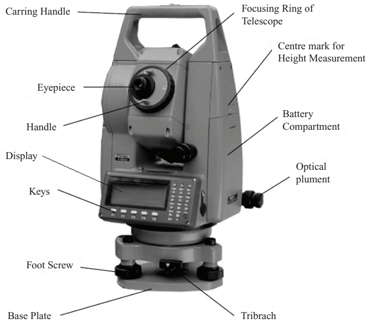
FIGURE 10.4 Parts of a total station
