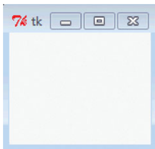
Figure 22.4 The tk window is opened when a tk file dialog command is called, but does not close when the dialog box is exited.
