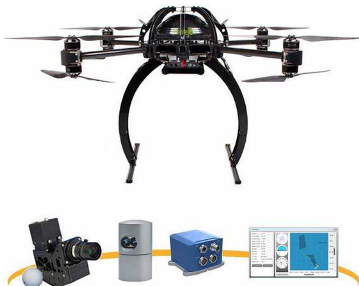
FIGURE 3.8 Typical components of a hyperspectral UAV.
