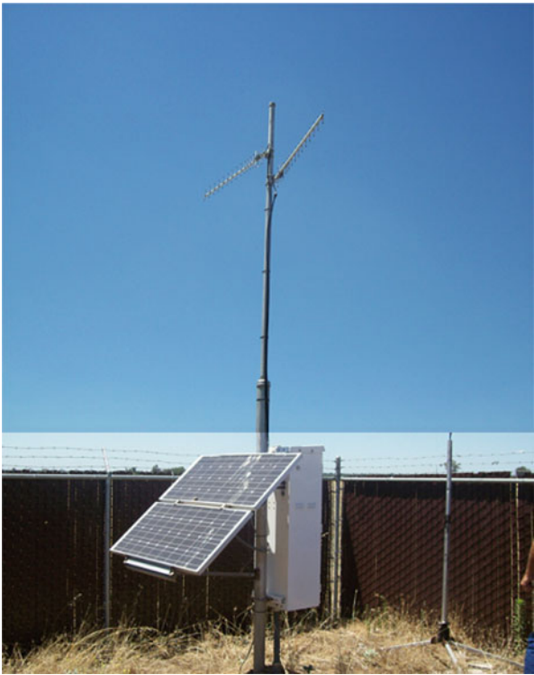
Fig. 6.3 GNSS CORS power supply and telemetry
