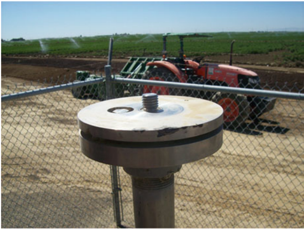
Fig. 6.4 Antenna mount without a GNSS antenna
