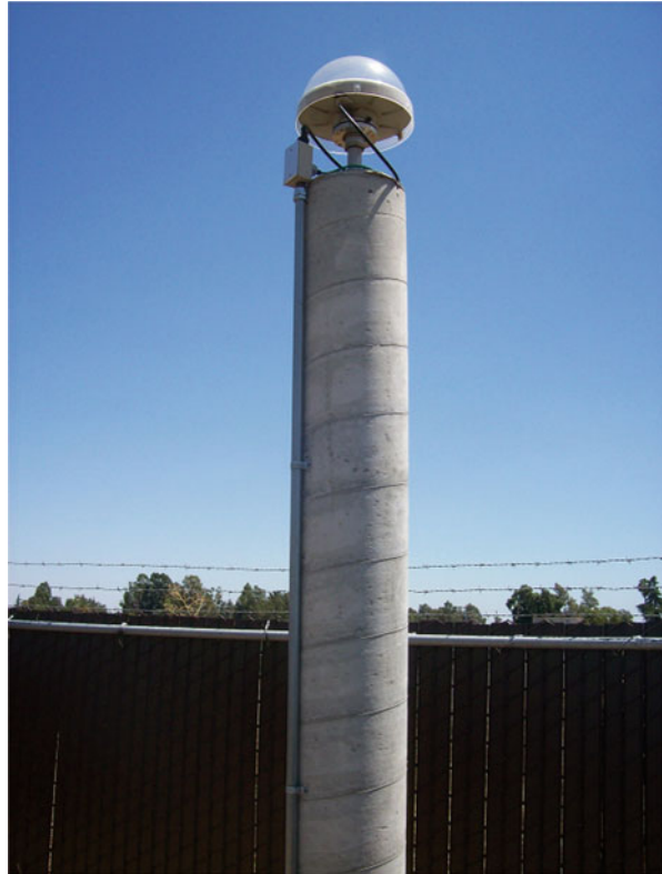
Fig. 6.1 GNSS CORS antenna on a monument pillar
