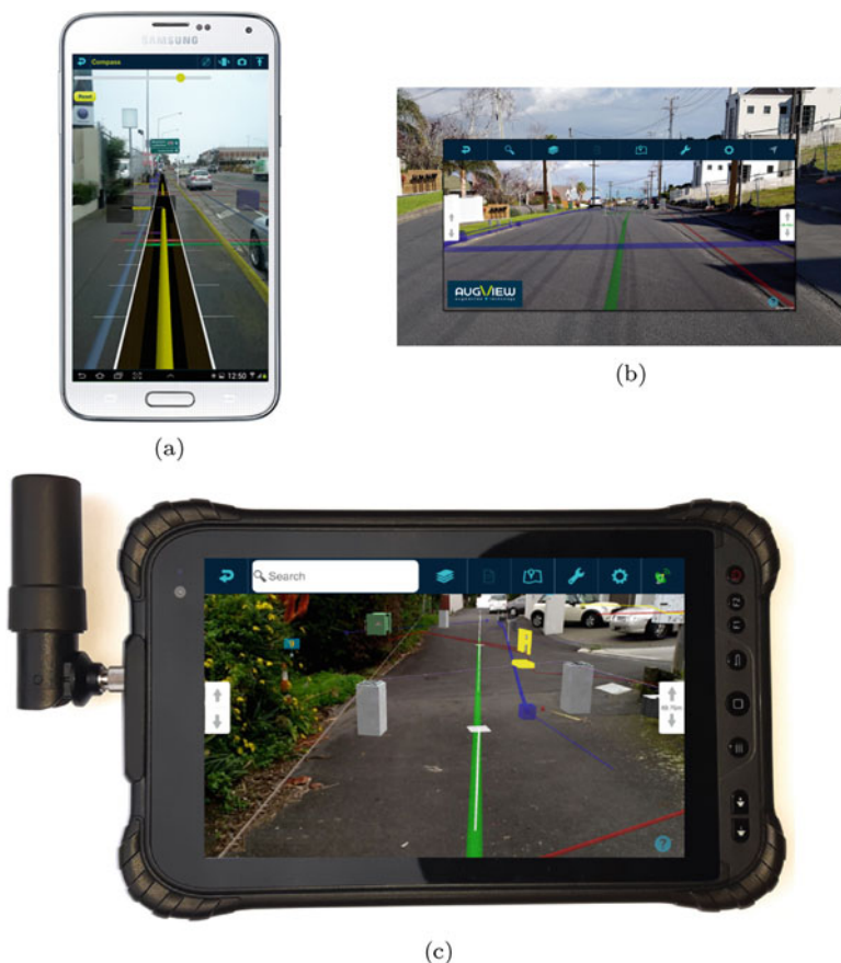
Fig. 1.1 Screenshots of augmented reality (AR) display systems. (a) AR on smartphone. (b) An AR of a street scene. (c) AR on ruggedized RTK tablet. Images used by permission. Courtesy of Augview Ltd
