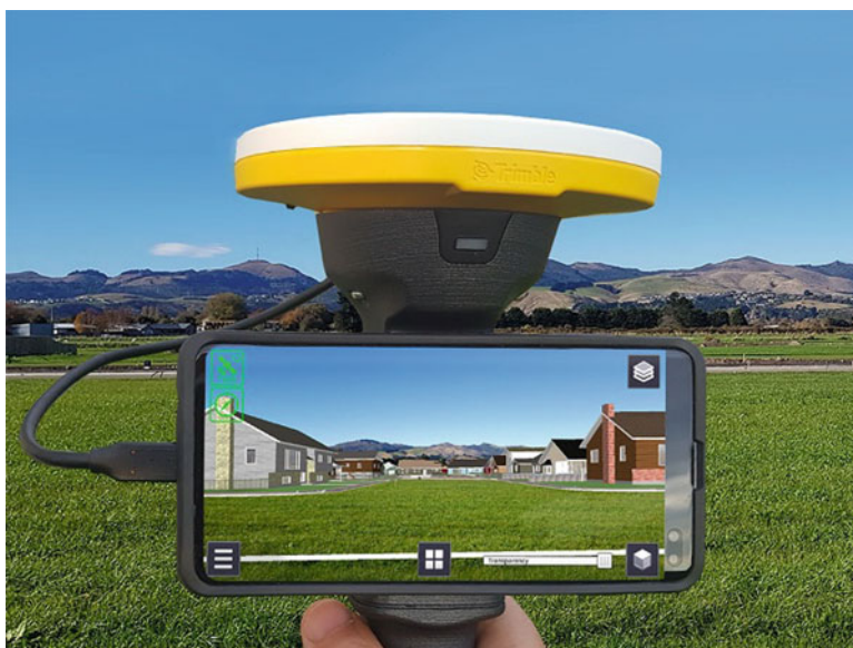
Fig. 1.2 A geodetic GNSS-based augmented reality system comprised of a geodetic antenna+receiver, data communication cable, and a mobile device with a display, camera, inertial orientation sensors, and other components. Image used by permission. Courtesy of Trimble Inc
