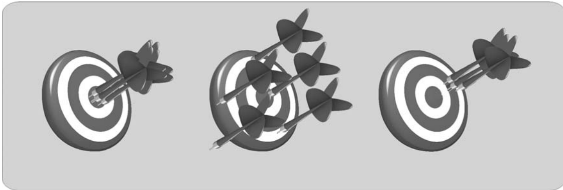
FIGURE 3.2: Accuracy and precision of an archer when the objective is to hit the center of the target in which good precision and good accuracy (left), bad precision and bad accuracy (center), and good precision and bad accuracy (right) are obtained.
