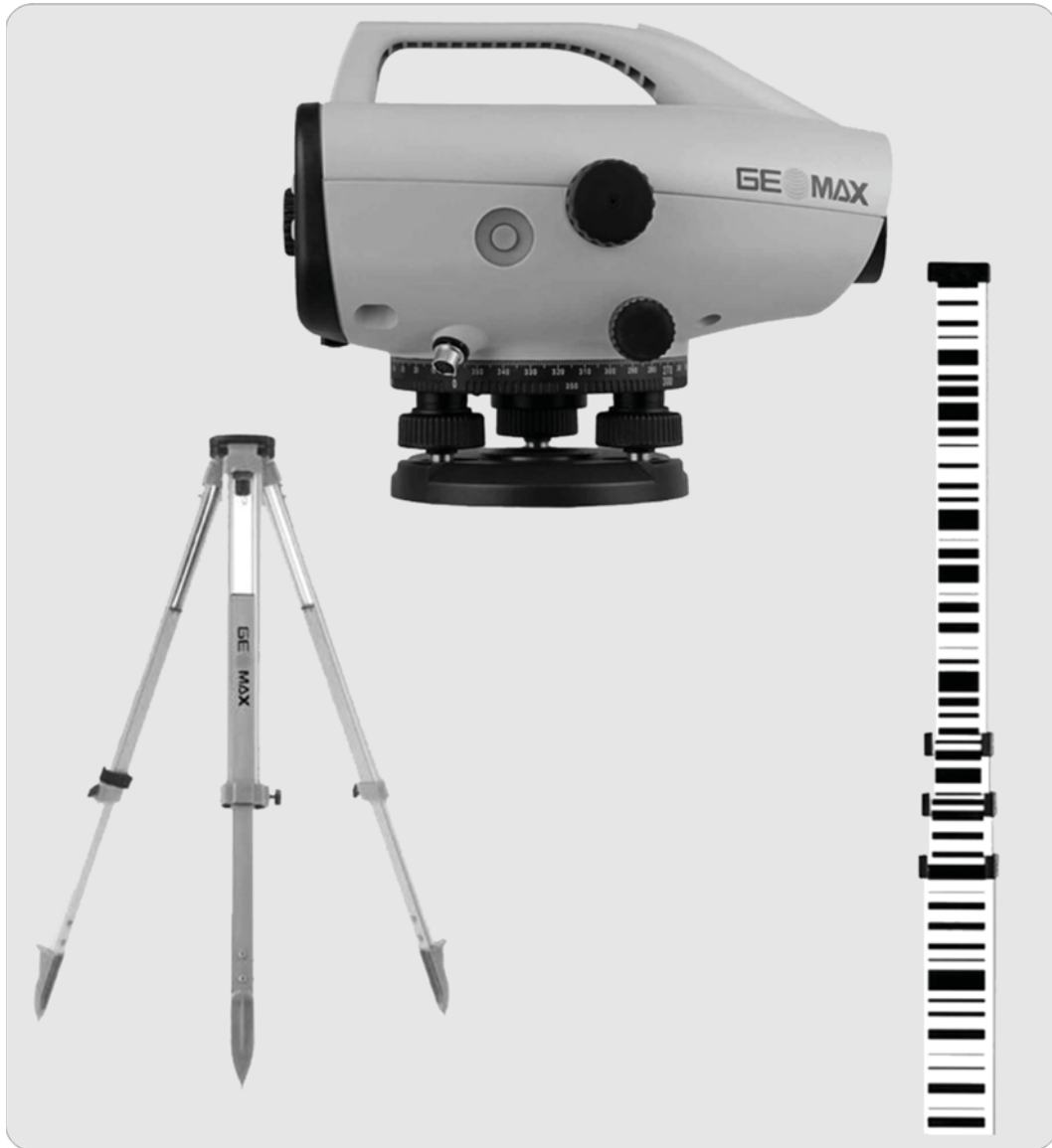
FIGURE 7.12: ZDL700 level with 3-second digital readout on double-sided levelling rod, accuracy of 0.7 mm per km, aluminum tripod.
