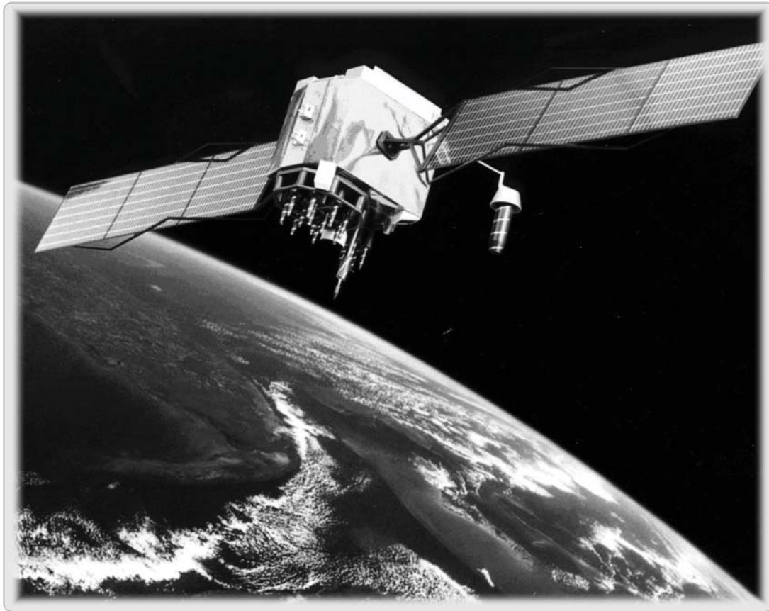
FIGURE 2.1: Artist's conception of global positioning system Block II-F satellite in Earth's orbit. (Courtesy of NASA.)
