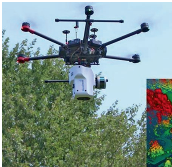
Fig. 22.4 VNIR/SWIR Hyperspectral spectrometer with integrated LIDAR for quantifying leaf wax and other unique heat stress adaptive traits
