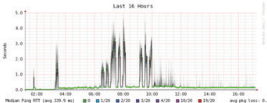
Figure 6.28: A higher spread of jitter is revealed in the 16 hour log.
