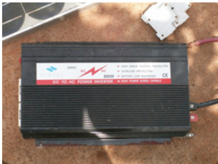
Figure 7.4: An 800 Watt DC/AC converter (power inverter)
