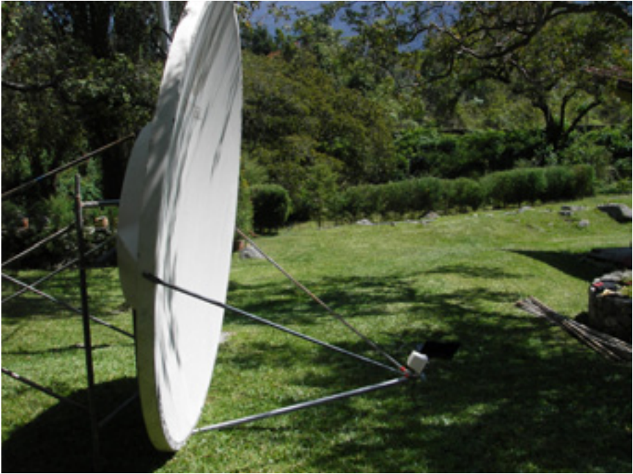
Figure 11.29: 2.4 m offset fed reflector with a 12 dBi antenna at its focus, looking 14° down. The actual elevation is 8° up.
