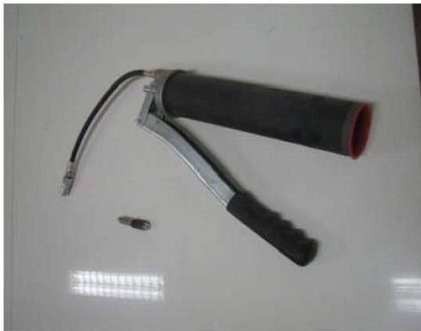
Figure 2. Packer and Injection Hand Pump
