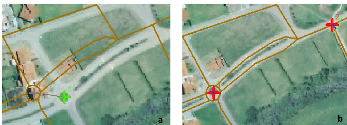
Figure 8. Georeferencing process, (a) initial linking point, (b) linked points
