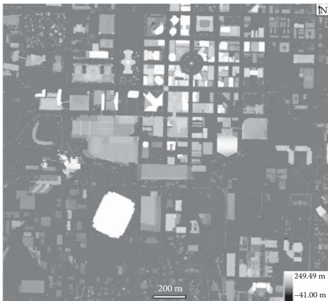
FIGURE 3.9 DHM raster created from DSM and DTM.
