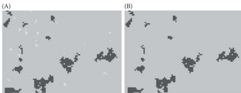
FIGURE 4.37 Removing selected foreground cells. (A) Connected cells less than four pixels are selected and (B) Selected foreground cells are erased.
