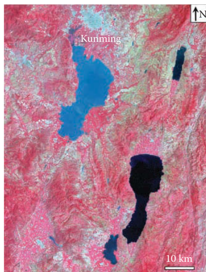
FIGURE 1.3 Color composite of Landsat-5 TM bands 4 (red), 3 (green), and 2 (blue) acquired on August 16, 1992, near Kunming, Yunnan, China.
