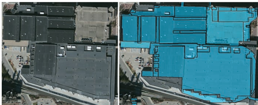
FIGURE 17.2 Step edge detection on a building roof.
