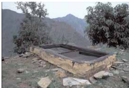
Figure 31: Mud dryer from Nepal © Practical Action.
