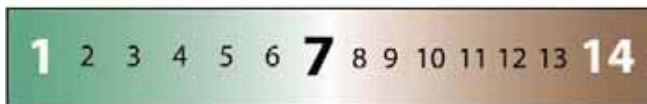
Figure 8: High acid foods have a low pH (below 4.5), low acid foods (alkali) have a high pH (above 5.3). A pH of 7 indicates neutrality.
