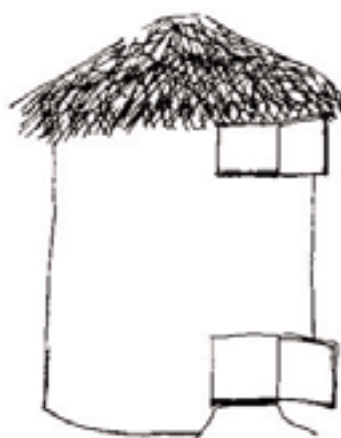
Figure 27: A cylindrical potato storage house.
