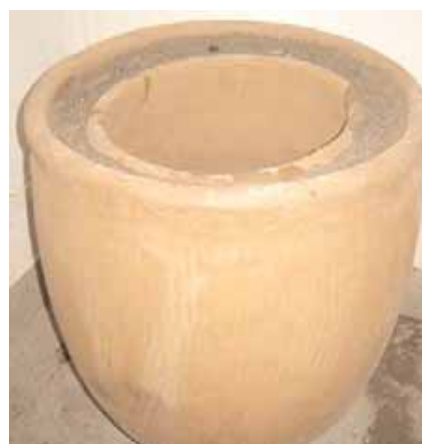
Figure 23. Example of a pot-in-pot cooler
