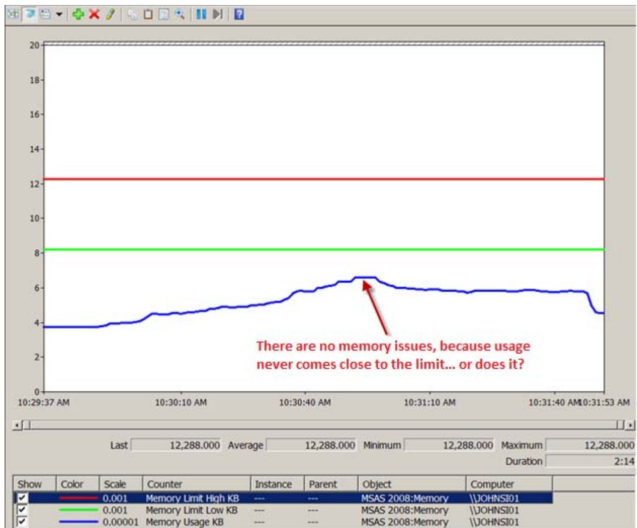
Figure 45 - Memory measurements with scaled counters
