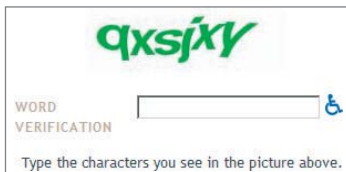
Figure 6-9: A CAPTCHA control designed to hinder automated attacks
