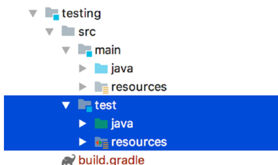
Figure 9-13. The Gradle module structure
