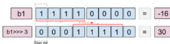
Figure 6-8. The effect of the >>> operator
