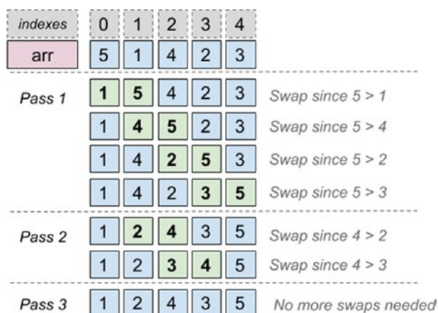
Figure 7-7. Bubble sort phases and effect
