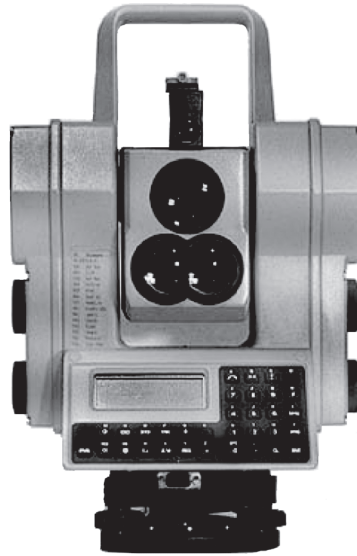
FIGURE 8.3 An old model total station
