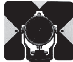
FIGURE 8.6 Typical standard prism and sight
