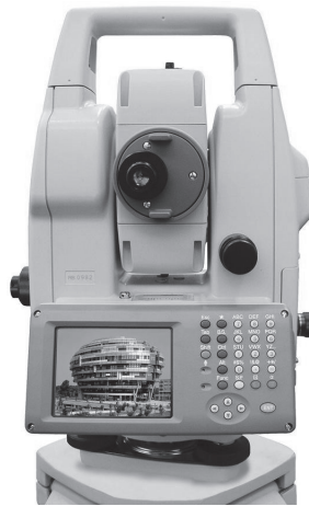
FIGURE 8.12 An imaging total station (courtesy of Sokkia)
