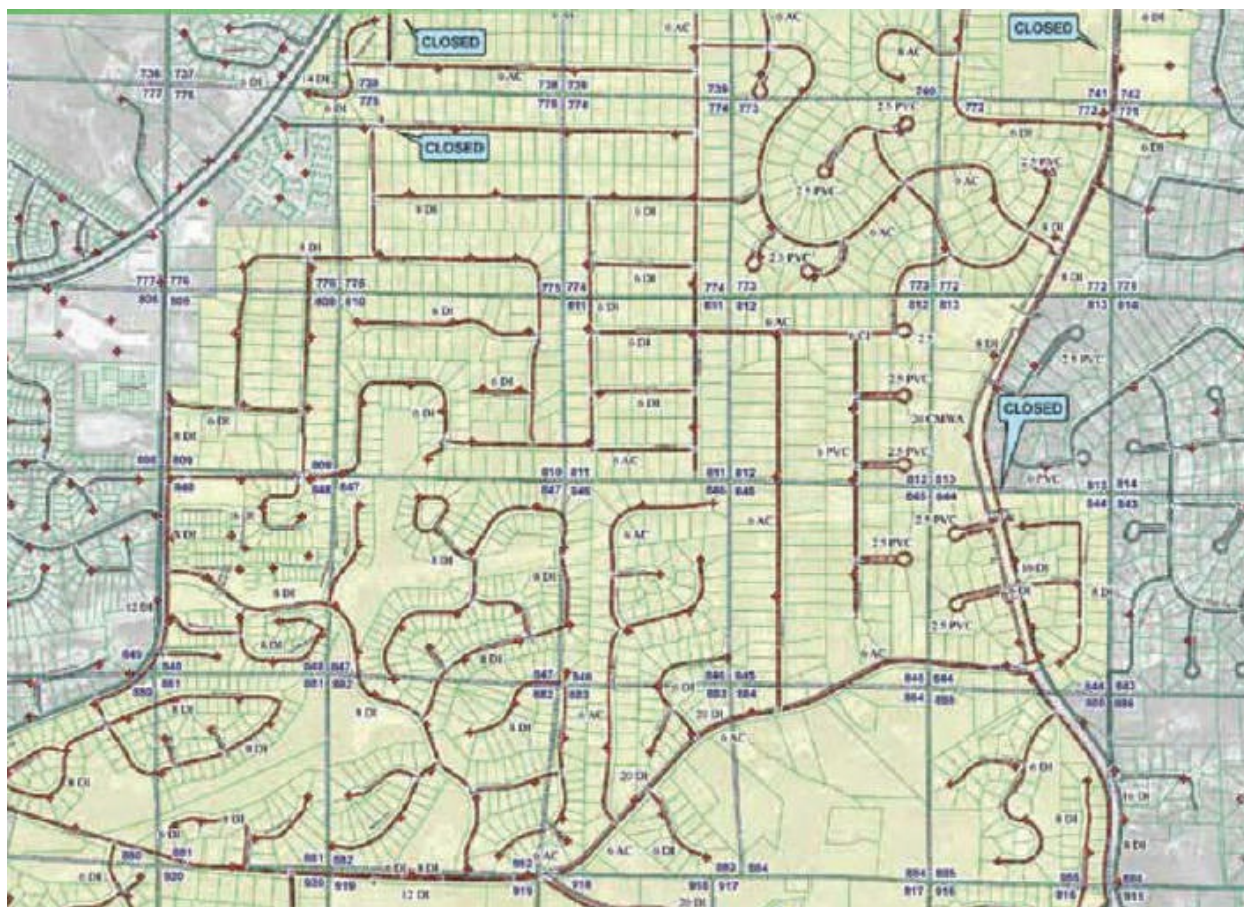
This utility map shows parcel locations, water lines, and valves for Cobb County Water System in Marietta, Georgia. Map courtesy of Cobb County Water System. Data from Cobb County GIS.
