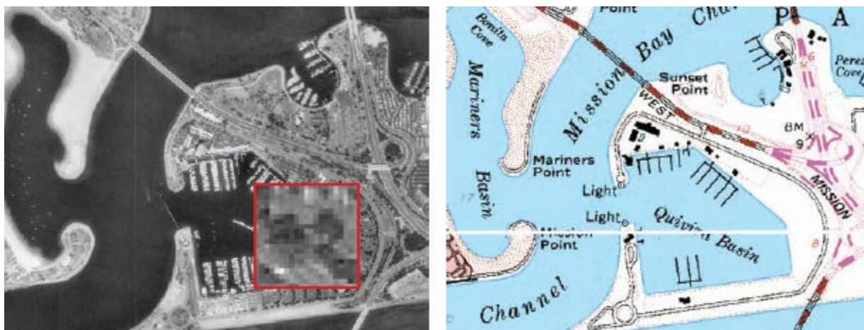
An air photo ( left ) and a scanned map ( right ) of the area around San Diego's Mission Bay. If you zoom in close enough on any raster, its cell structure will be revealed, as shown by the inset in the red box on the air photo. Satellite image and map courtesy of the US Geological Survey.
