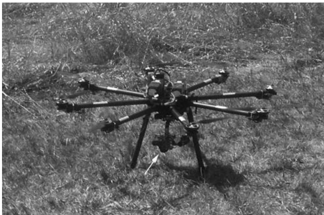
FIGURE 12.2 UAV and camera. The arrow shows the camera mounting at the bottom of UAV.
