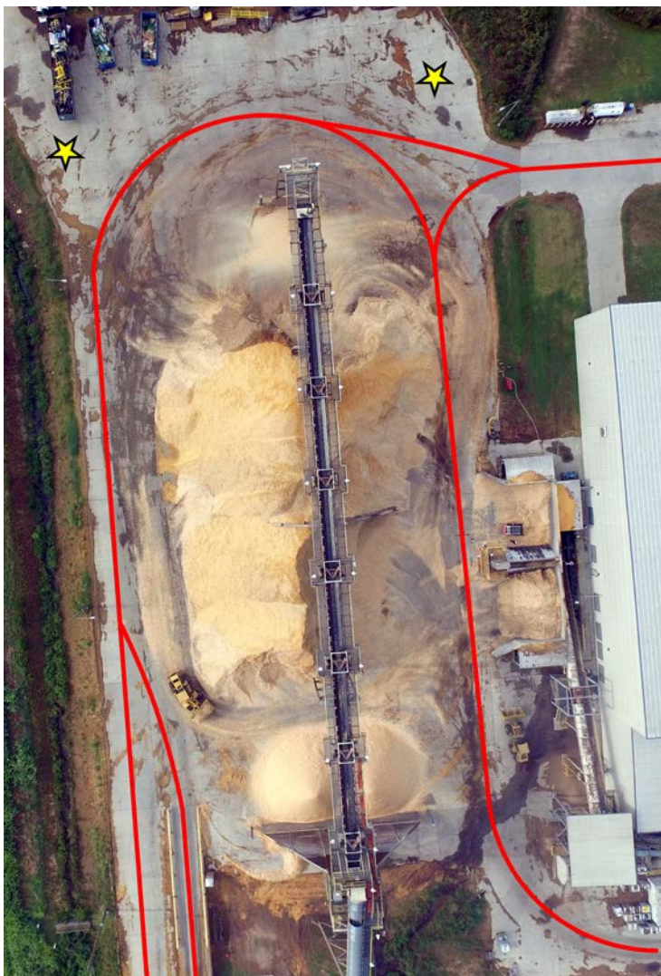
FIGURE 7.3 Mosaic generated using Agisoft PhotoScan of the study site, with an overlay of UAS pilot positions (star) and equipment traffic areas (thick line).
