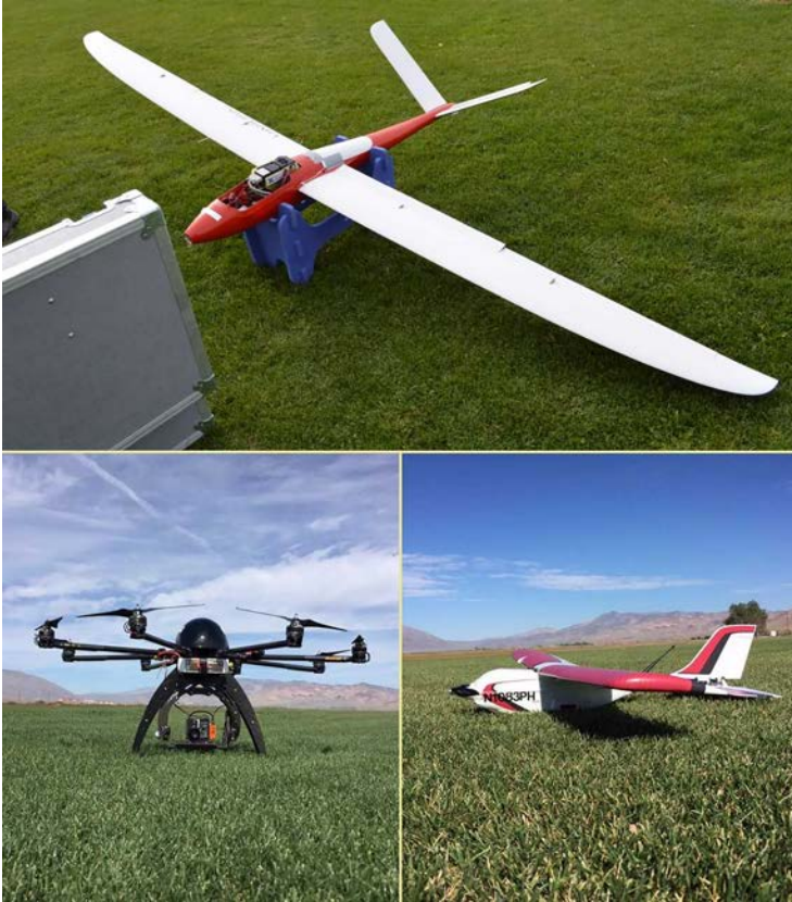
FIGURE 3.9 Examples of fixed-wing and octocopter hyperspectral UAVs.
