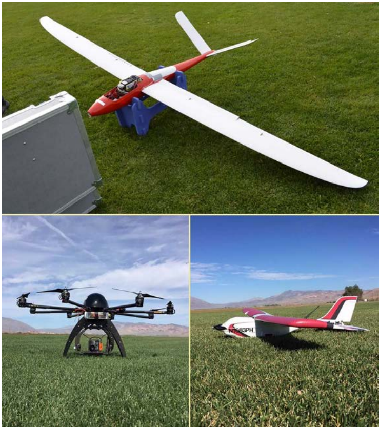
FIGURE 3.9 Examples of fixed-wing and octocopter hyperspectral UAVs.
