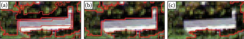
FIGURE 10.3 Segmentation results at scales of (a) 30, (b) 50, and (c) 70.
