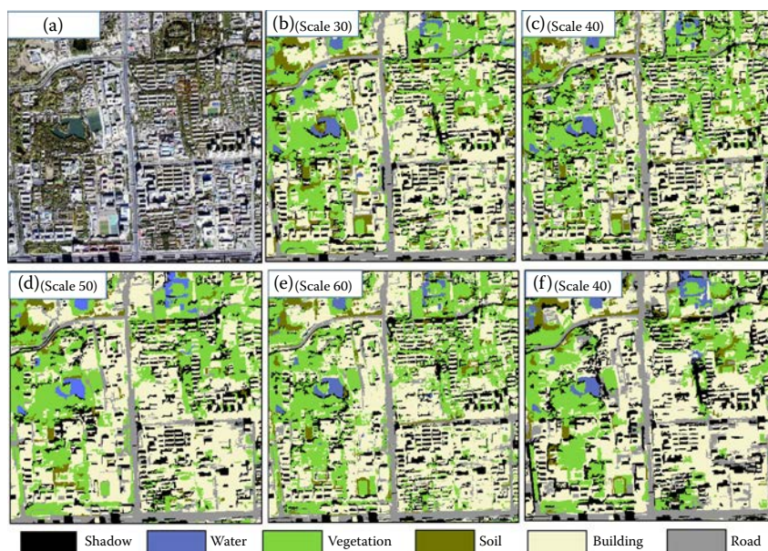
FIGURE 10.12 Object classification results of the (a) WorldView-2 image at (b–f) five scales. (From Zhang, X., & Du, S. 2016. Remote Sensing of Environment , 178, 172–190.)
