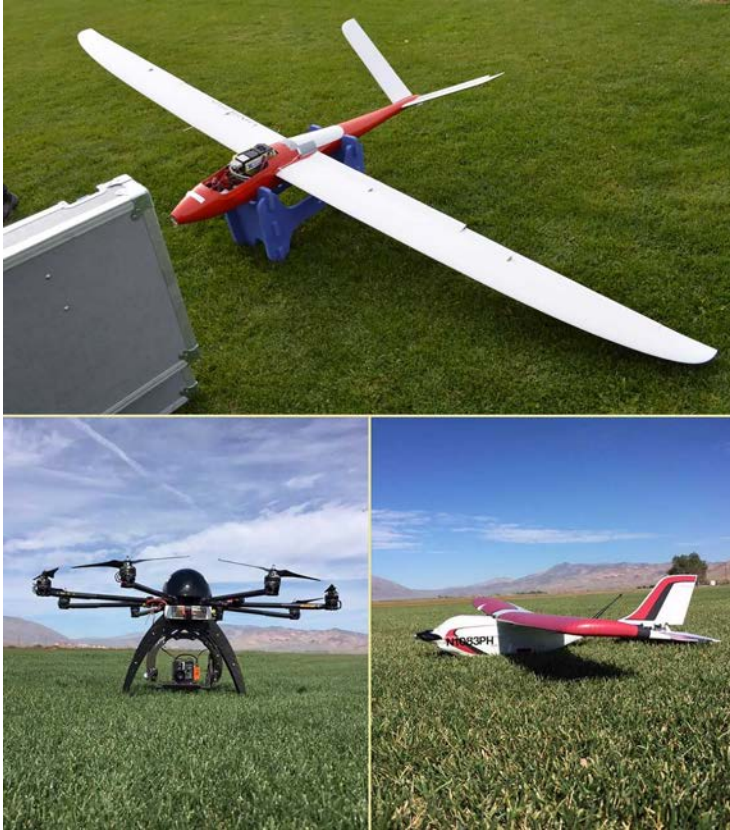
FIGURE 3.9 Examples of fixed-wing and octocopter hyperspectral UAVs.
