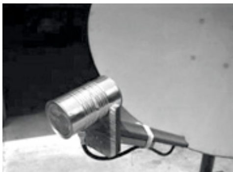
Figure 4.10: Feed horn made from a food can.
