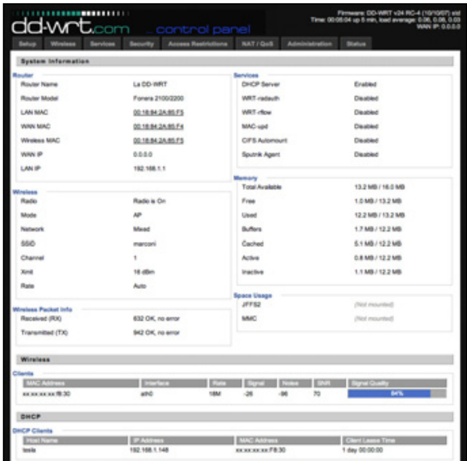
Figure 5.3: The DD-WRT (v23) control panel
