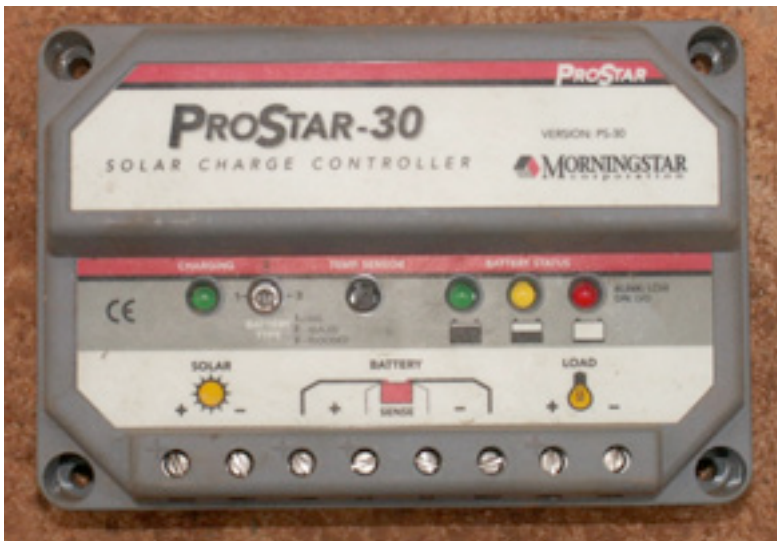
Figure 7.3: A 30 Amp solar charge controller
