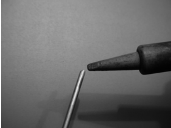
Figure 4.37: Tin the end of the wire before soldering.
