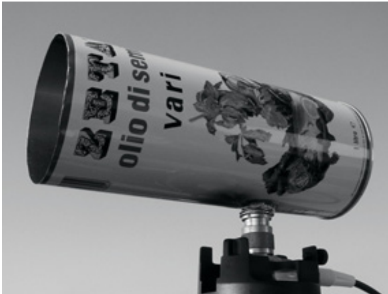
Figure 4.32: The finished cantenna.
