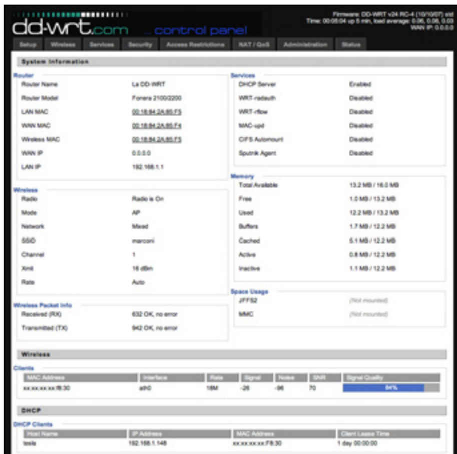
Figure 5.3: The DD-WRT (v23) control panel
