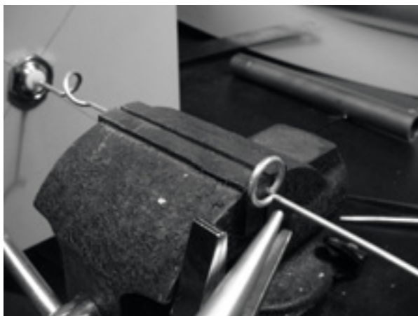
Figure 4.28: Repeat the stretching procedure for all of the remaining coils.
