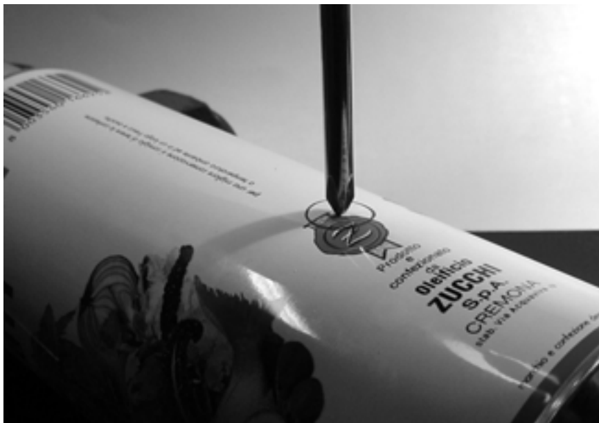
Figure 4.35: Mark the hole before drilling.
