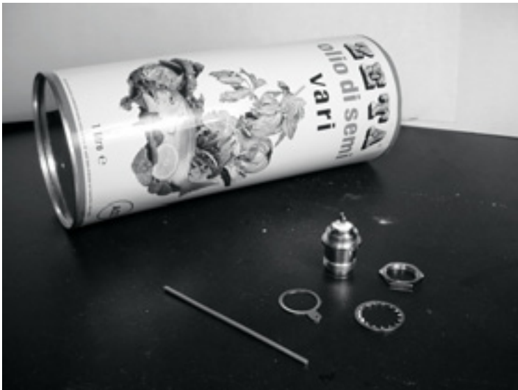
Figure 4.33: Parts needed for the can antenna.
