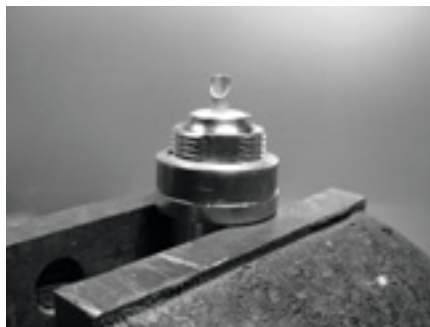
Figure 4.23: Adding a copper pipe spacer helps to match the impedance of the antenna to 50 Ohms.
