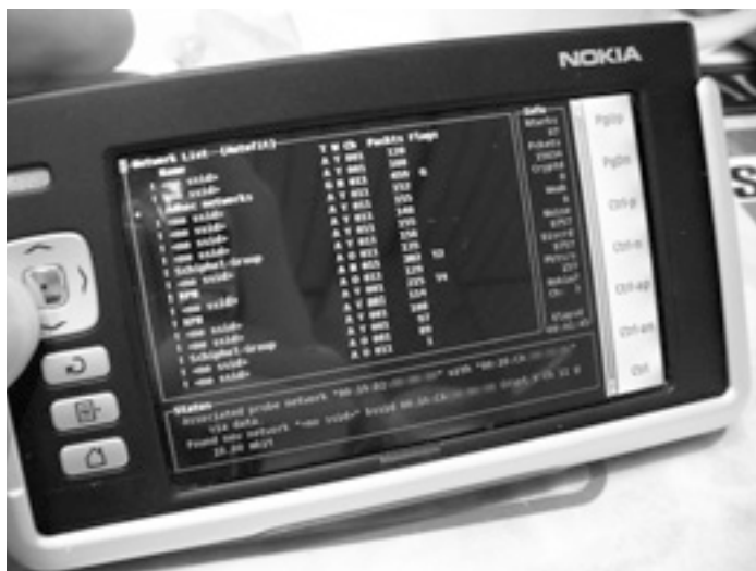
Figure 6.12: Kismet running on a Nokia 770 Internet Tablet
