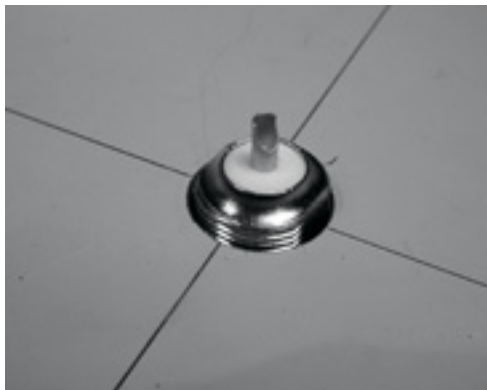
Figure 4.22: The N connector should fit snugly in the hole.
