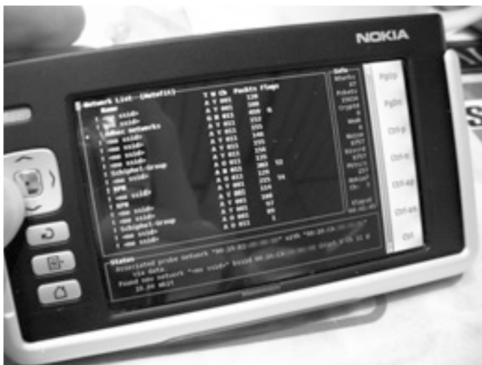
Figure 6.12: Kismet running on a Nokia 770 Internet Tablet
