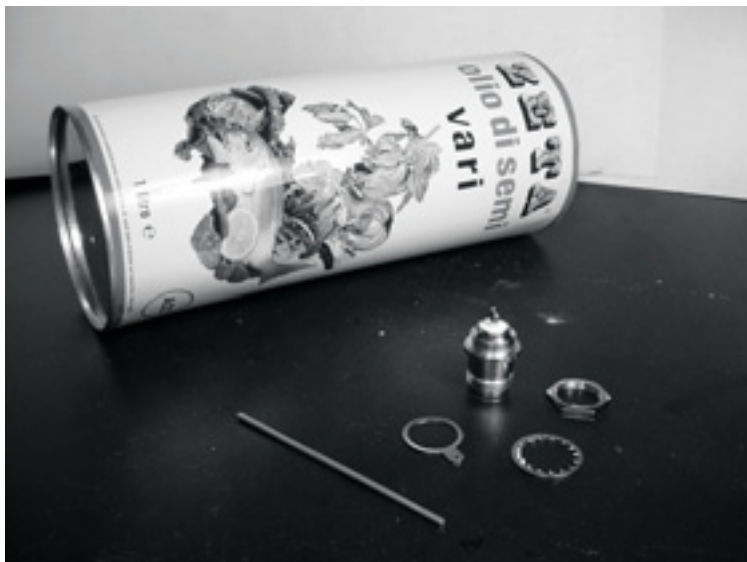
Figure 4.33: Parts needed for the can antenna.
