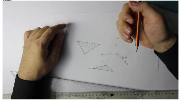
You first need to have the triangle constructed in a triple projection, then copy the length of the vertical edge and of the height in axonometric and then connect the three dots adjacent to get an even triangle.
