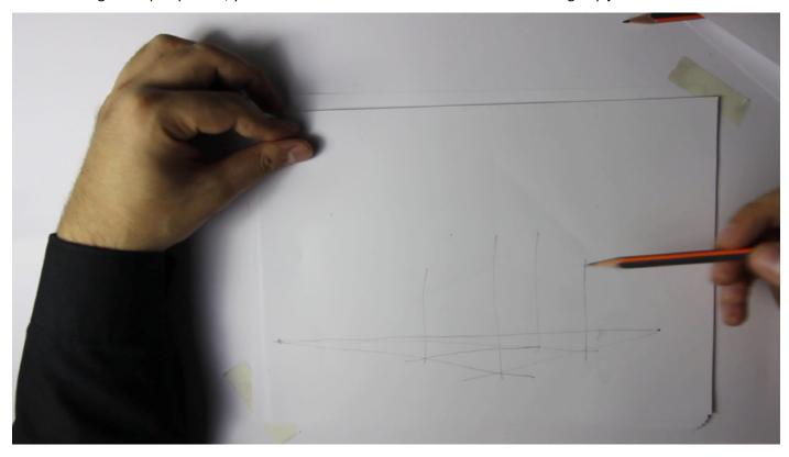
Just remember, you need to measure the height of the box on its closest edge - this way you will have an accurate measurement of the perspective height.
