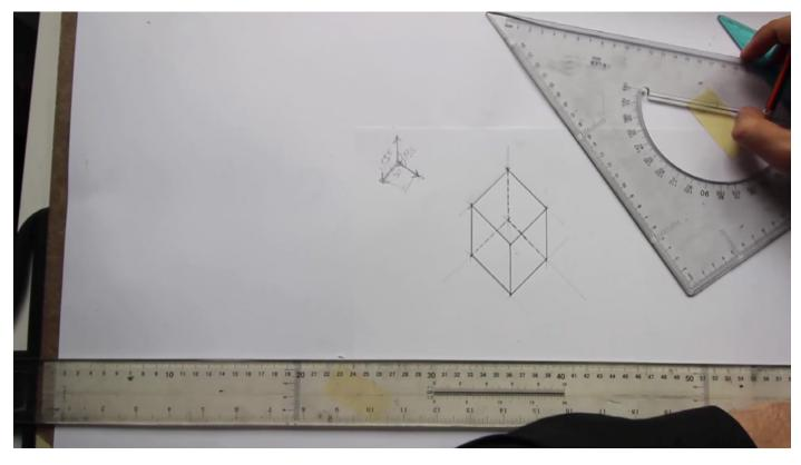
The Ox axis also has a half the unit the other two axes have... since the name di-metric, meaning two different measurements and units.
