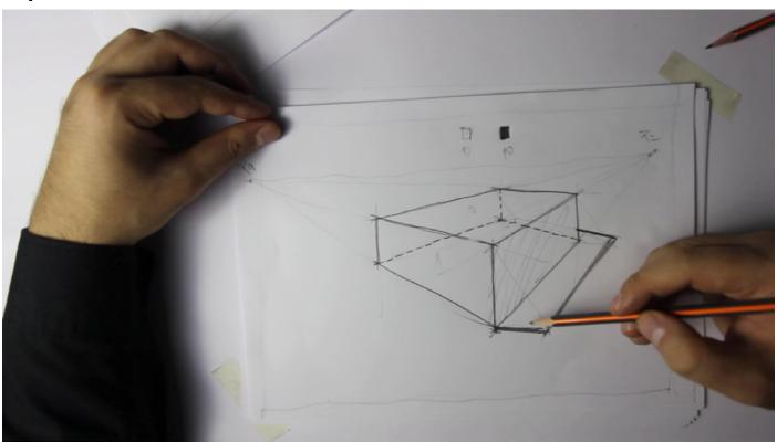
Hatching a top-down perspective is really simple: just construct an estimated cast shadow on the short side, then hatch the shadowed face adjacent to the cast shadow.
