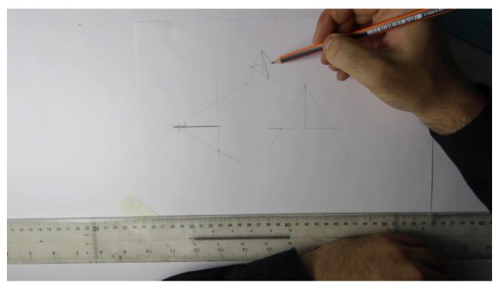
Then from one of theend of the vertical edge draw an arch with the same length as the edge and intersect it with the height on the right-hand side.
