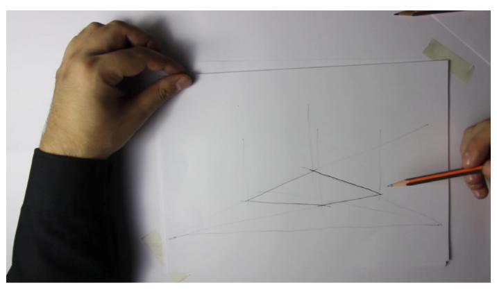
Then we will go for drawing heights and are the mirrored line construction of the standard top-down perspective... the only difference being that you start with constructing the bottom of the box and you move up from there, in con-
