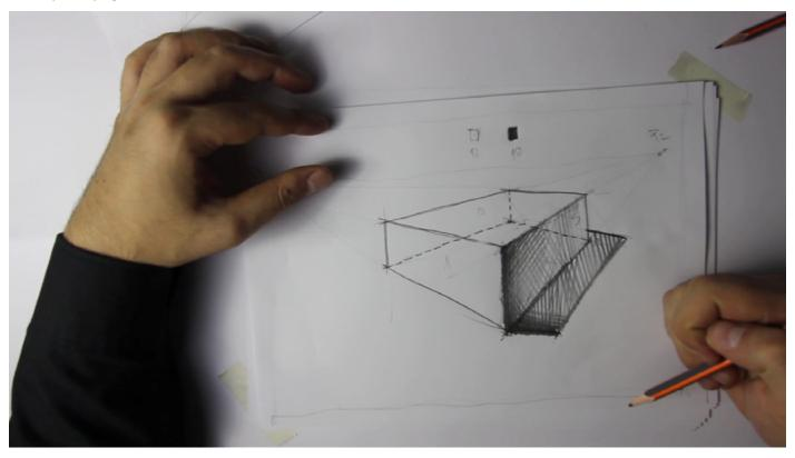
Also, the intensity of the cast shadow should be 10 to 8 (according to how close the shadow is in perspective), and that of the shadowed face should vary from 5 to 3, following the same rationale.
