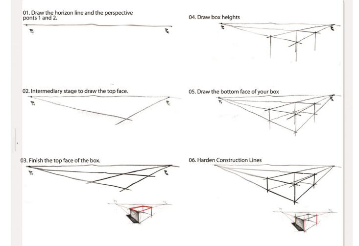
These above six steps are the fundamentals for drawing any two-point perspective.
