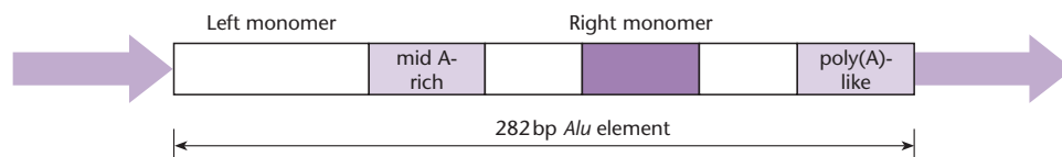
Fig. 16.19 Structure of a typical 282-bp Alu element flanked by direct repeats (purple arrows). The Alu element itself consists of an inexact duplication of two monomer units separated by a mid A-rich region. The right monomer contains an additional sequence of approximately 30 bp (dark green) that is absent from the left monomer. The consensus sequence usually is followed by an A-rich region resembling a poly(A) tail.
