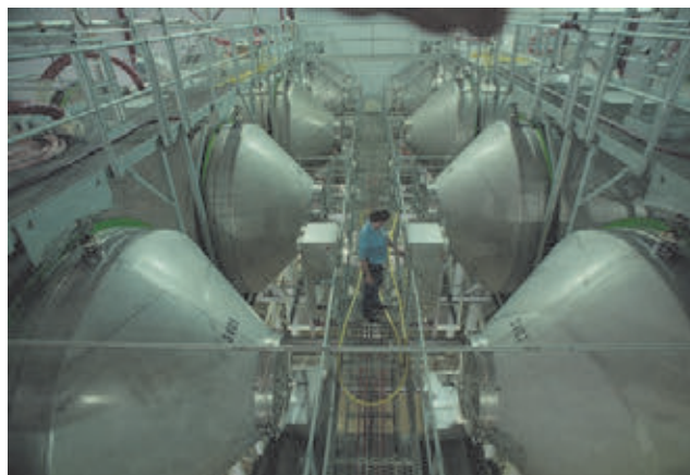
FIGURE 1 Industrial-scale fermentations to produce biofuel and other products are typically carried out in tanks that hold thousands of liters of medium.
